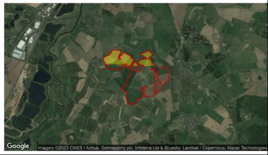
Observer Location Sun azimuth range is 270° - 288.2° (yellow)
